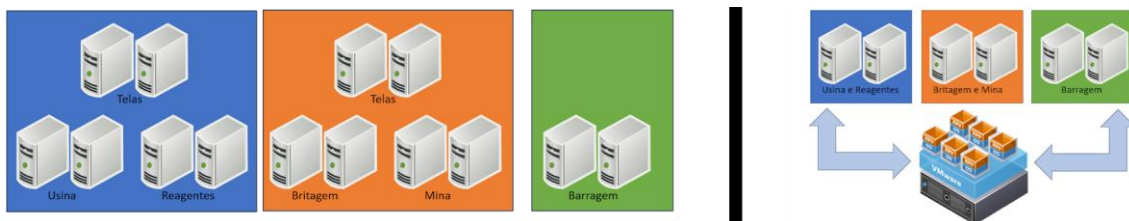
Samarco's former and current SCADA system architecture
