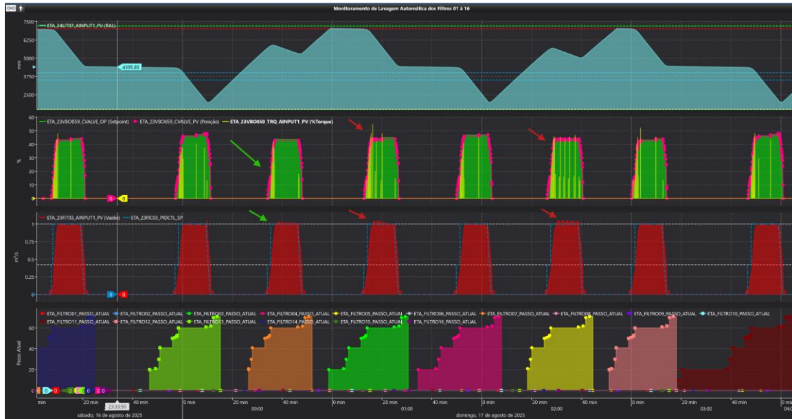
Torque-controlled loops: One regular (green arrow) and two out of order (red arrows), causing fluctuations in the flow control at the WTP
