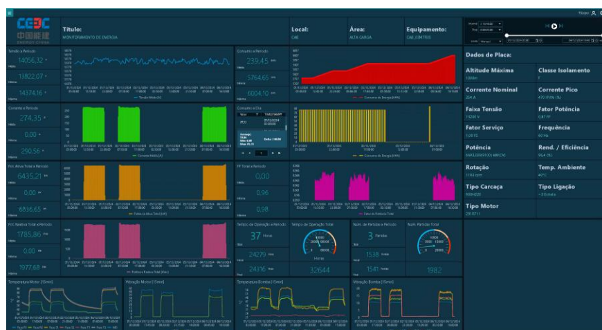
EPM charts for monitoring the operating variables of the pump motors at the RWI
