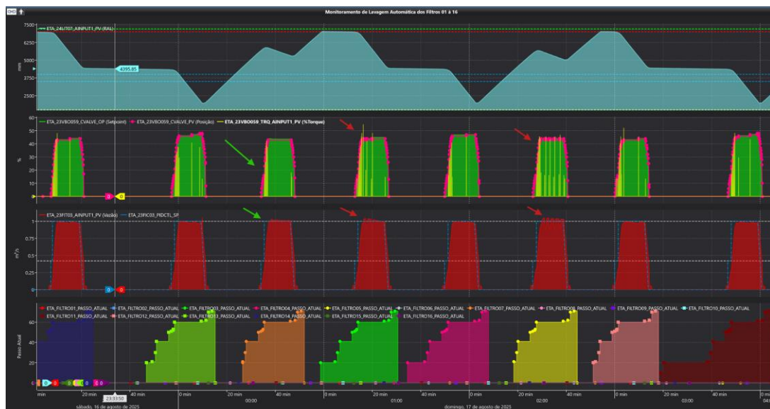
One control cycle with a normal torque reading (green arrows) and two cycles with abnormal torque readings (red arrows), causing fluctuations in flow control at the WTP
