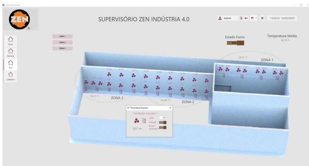
Elipse E3's screen for controlling furnace and exhaust fans at the ZEN plant pavilion
