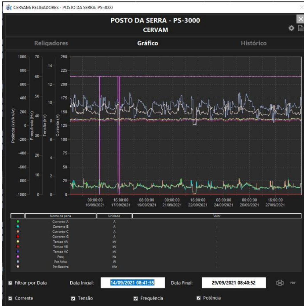
Figure 3. Graphic sample of a recloser's current, power, and frequency
