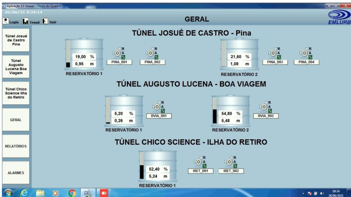
*Water levels control at tunnels' reservoirs*
