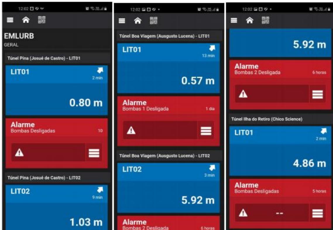
*Elipse Mobile screens monitor the level at reservoirs and turned off pumps*
