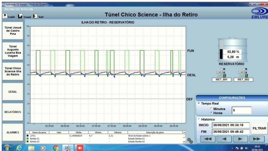
**Screen charts depicting pumps and water level at reservoirs from Chico Science tunnel's drainage system**
