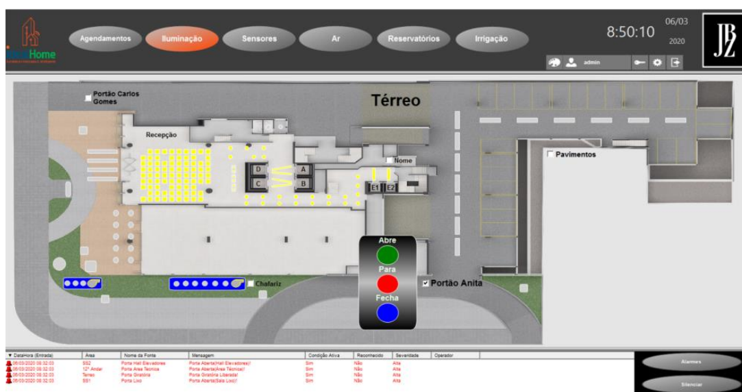
Figure 2. Lights, irrigation, and parking lot gates control at the ground floor
