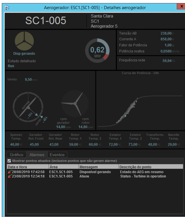
Figure 4. Control screen of a wind turbine at Santa Clara Wind Park
