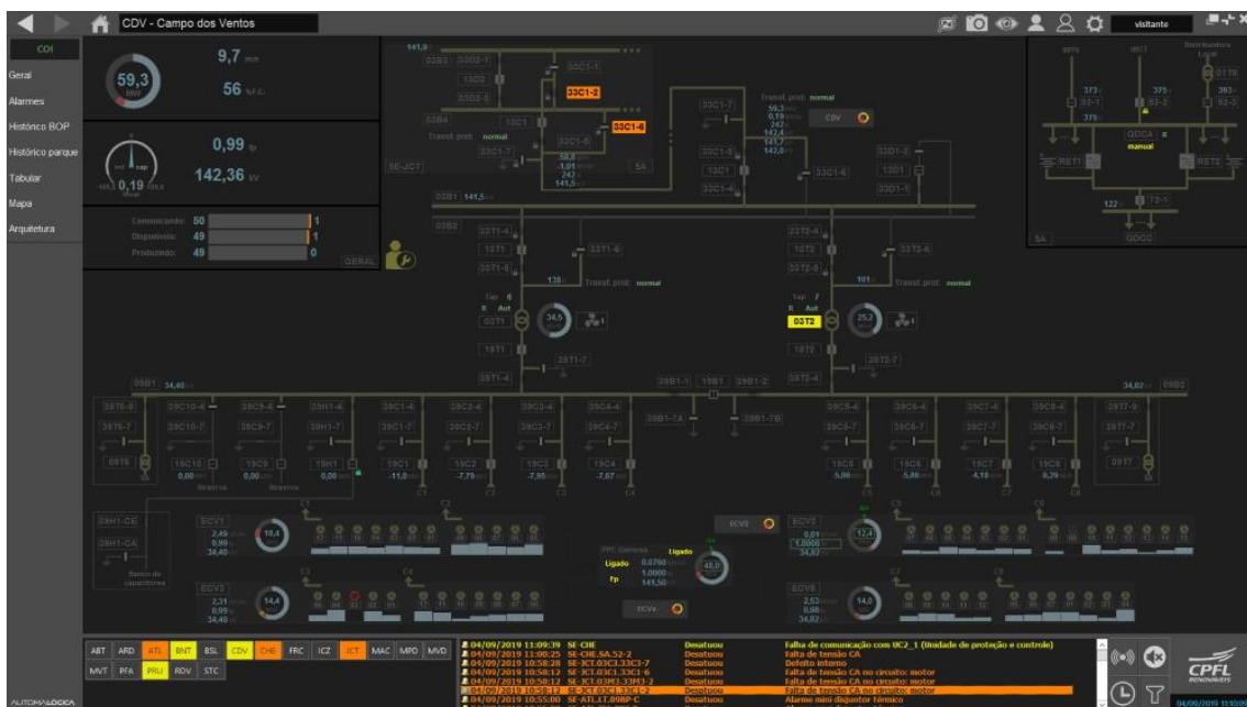
Figure 3. Elipse Power Renewable screen monitoring Campo dos Ventos Wind Complex
