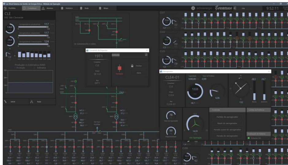
Figure 5. São Clemente Complex control via Elipse Power
