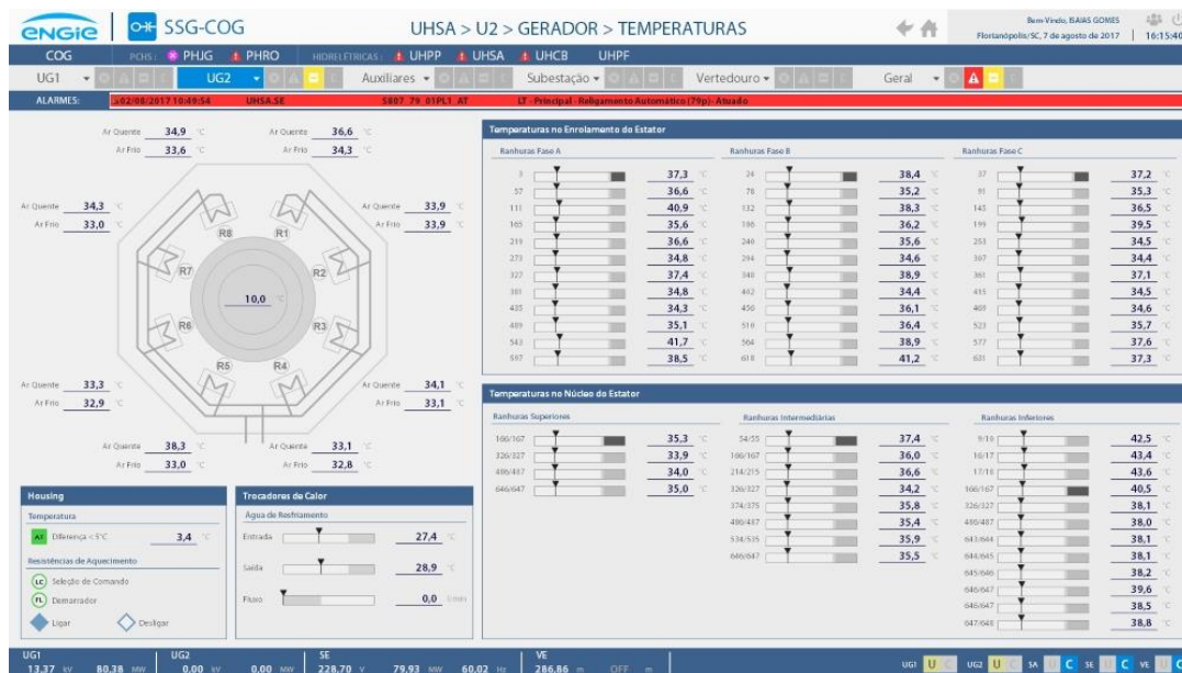
Figure 4. Windings and slots control
