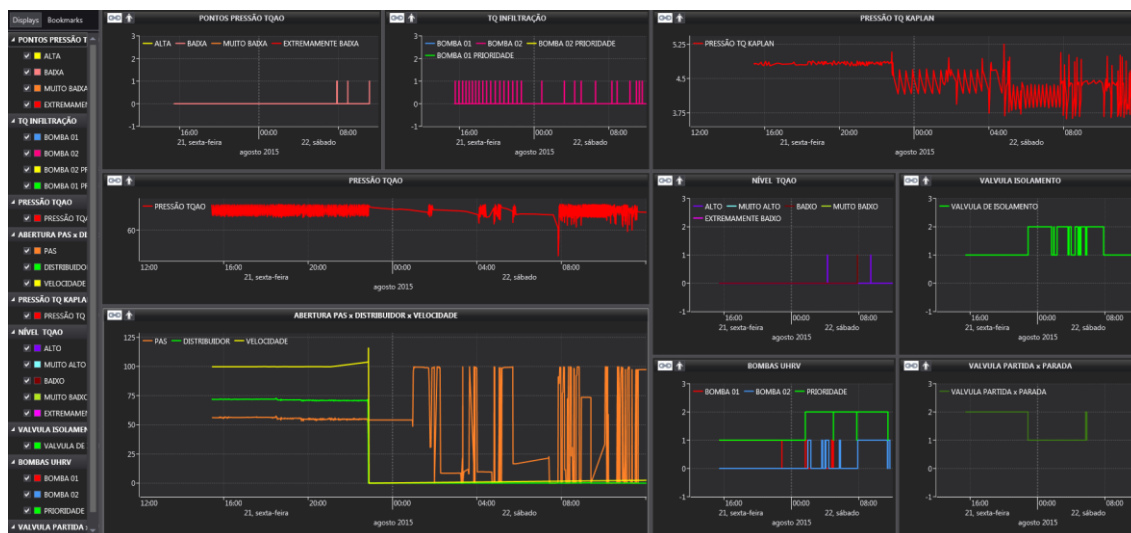
Figure 2. EPM screen used to analyze the hydraulic unit of the speed regulator of generator units
