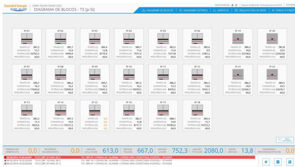
Figure 7. Set of inverters associated to the polycrystalline silicon boards
