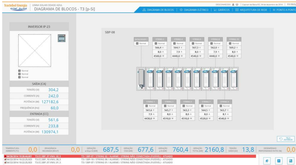
Figure 8. IP-23 inverter's monitoring screen related to 10 strings
