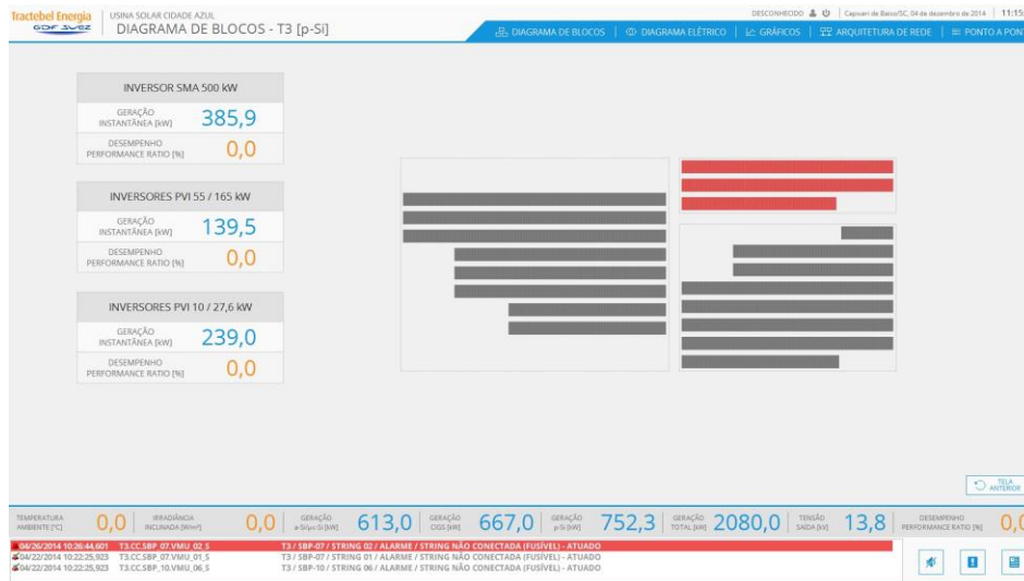
Figure 6. Screen displaying the energy generated by polycrystalline silicon boards with three different inverters, with 10, 165, and 500 kW
