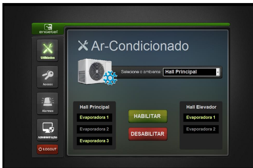
Screen to control the air conditioning located on the building's main hall
