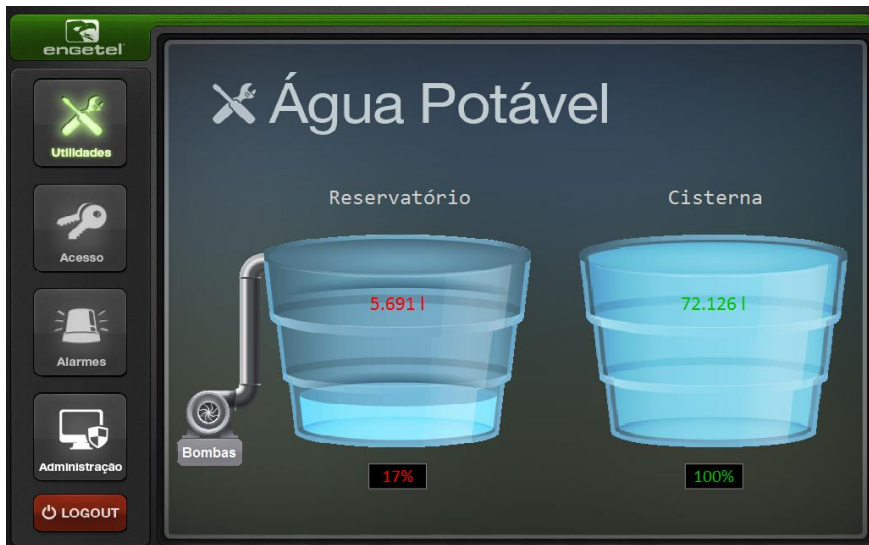
Screen to control levels of water in the tank and in the reusable cistern
