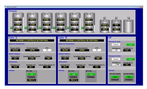
Figure 2. Control screen in the plant's reception
