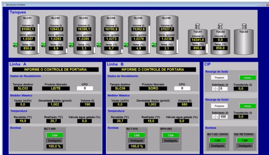
Figure 2. Control screen in the plant's reception
