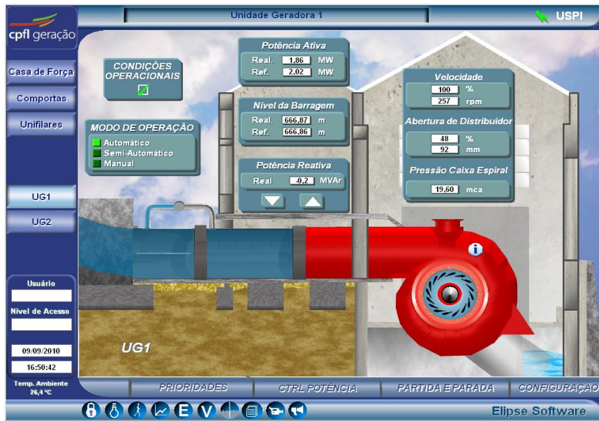
Figure 6. Screen displaying the opening percentage of the distributor's blades
