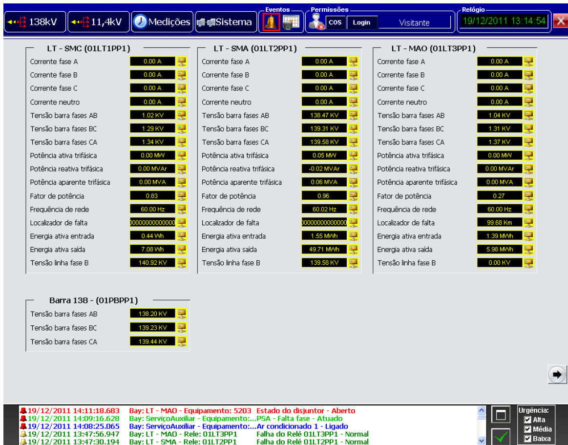
Figure 6. Screen displaying a few measurements signaled with the substation
