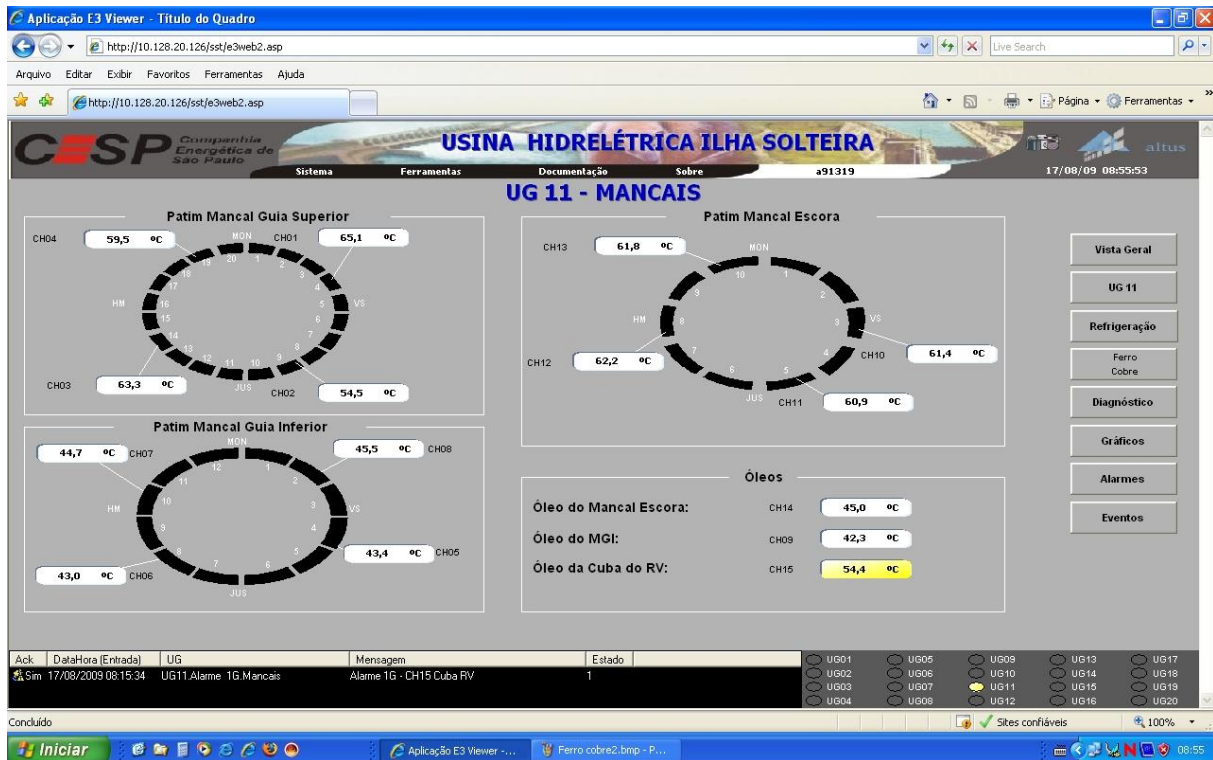
Figure 6. Screen monitoring temperature in bearings
