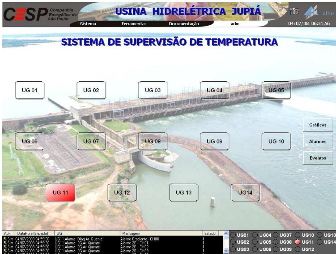
Figure 1. Initial screen of the monitoring system in UHE Jupiá’s generating units
