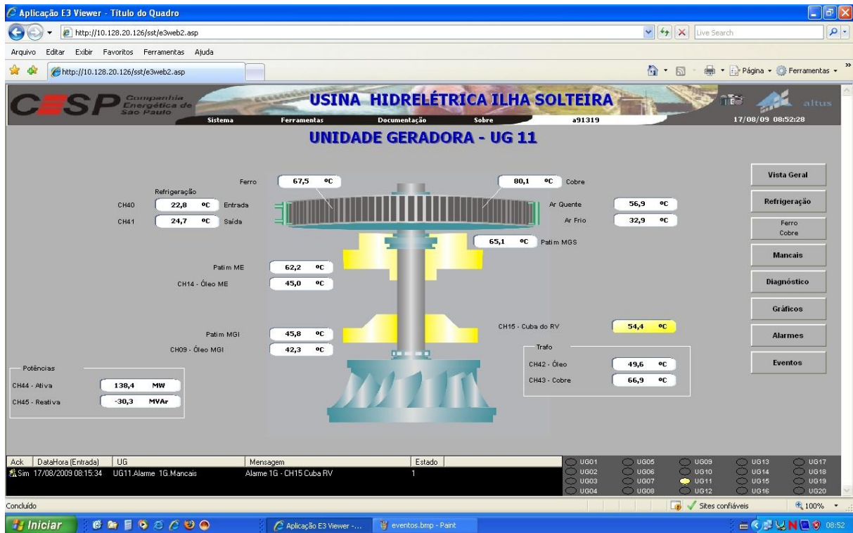
Figure 4. Screen displaying temperatures recorded in one of UHE Ilha Solteira’s generating units
